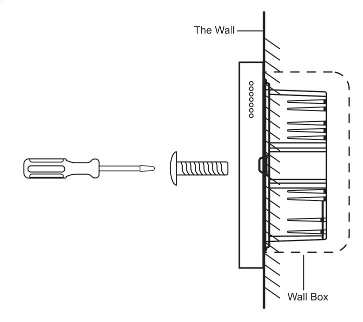
Note: Depth of the wall box must be more than 50mm.
